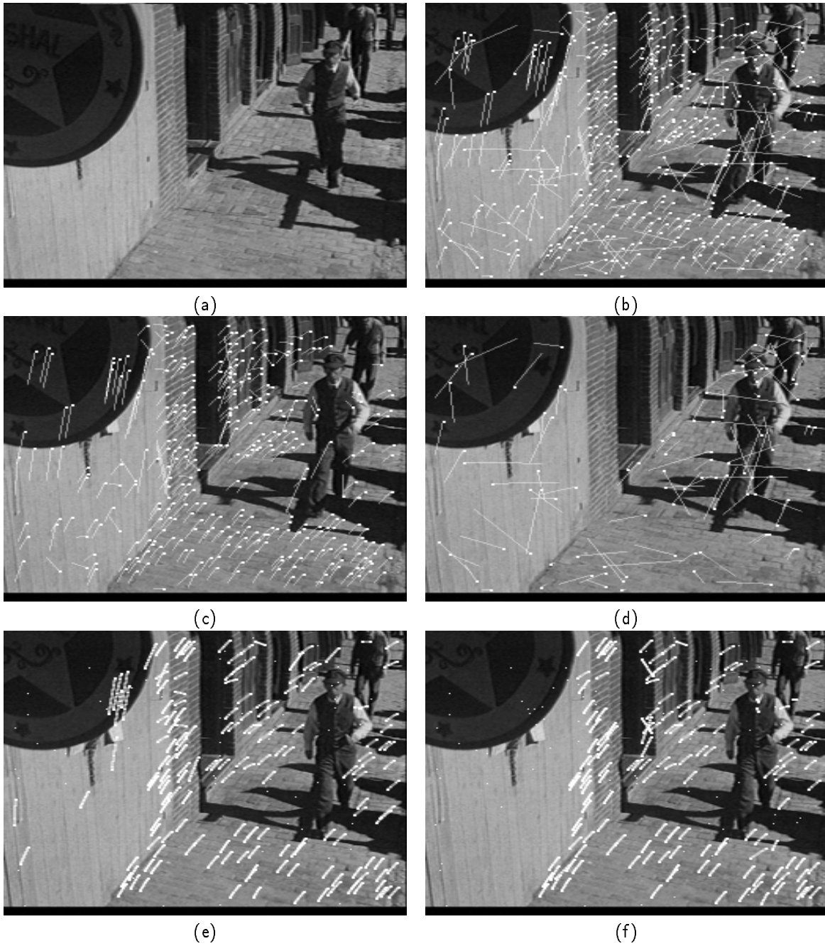
Fig. 16. Two images from a sequence showing the movement of a person towards the camera as the camera moves to keep him in view, with the resulting correspondences from corner matching in (b). The combined RANSAC/Huber M-estimator segments the set of correspondences into (c) inliers and (d) outliers. (e) inliers from M-estimator. (f) inliers from case deletion diagnostic.
