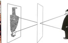
subject got through the tiny opening, producing a soft but acceptably clear photograph. Because of the small size of the pinhole, the exposure had to be 6 sec. long.
