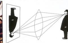
The lens opening was much bigger than the pinhole, letting in far more light, but it focused the rays from each point on the subject precisely so that they were sharp on the film.
