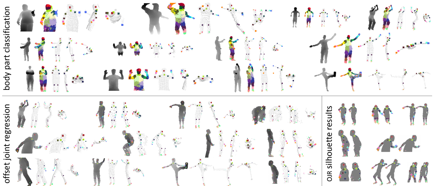
Fig. 10. Example inferences on both synthetic and real test images. In each example we see the input depth image, the inferred most likely body part labels (for BPC only), and the inferred body joint proposals shown as front, right, and top views overlaid on a depth point cloud. Only the most confident proposal for each joint above a fixed, shared threshold is shown, though the algorithms predict multiple proposals per joint. Both algorithms achieve accurate prediction of body joints for varied body sizes, poses, and clothing. We show failure modes in the bottom rows of the two larger panels. There is little qualitatively to tell between the two algorithms, though the middle row of the OJR results shows accurate prediction of even occluded joints (not possible with BPC), and further results in Sec. 4.6 compare quantitatively. Best viewed digitally at high zoom.
