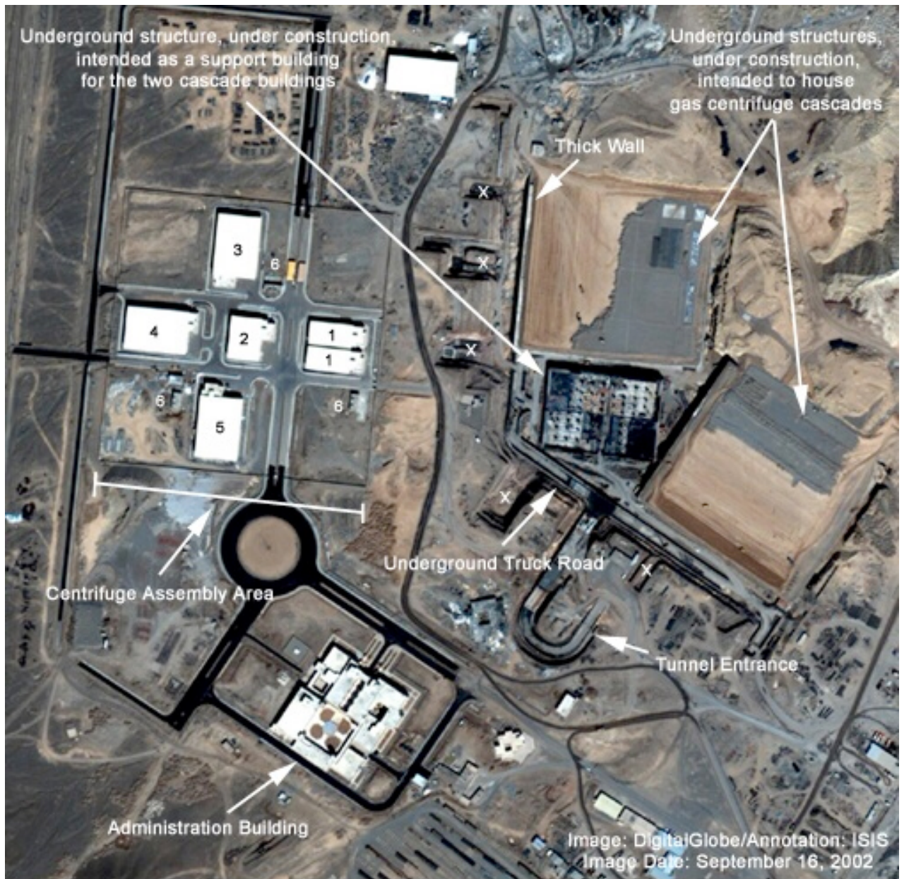
Satellite image of the Natanz nuclear enrichment plant in Iran taken in 2002 when it was still under construction. The image shows two cascade halls, in the upper right corner, as they were being built deep underground. The hall on the
