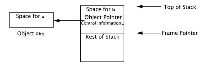
When **a+b** is computed, **b**, a local variable, is accessed directly through the frame pointer. **a**, a member of object **obj**, is accessed indirectly through the object pointer that is stored in the frame (as all parameters to a method are).
