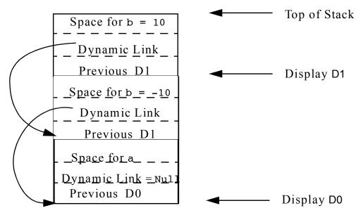
Since q is at nesting level 1, its frame is pointed to by D1. All of q's local variables, including b, are at a fixed offset relative to D1.
