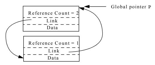
set to null, the object's reference count is reduced to 1. Both objects have a non-zero count, but neither is accessible through any external pointer. The two objects are garbage, but won't be recognized as such.
