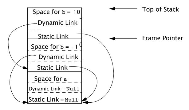
As usual, dynamic links always point to the next frame down in the stack. Static links always point down, but they may skip past many frames. They always point to the most recent frame of the routine that statically encloses the current routine.
