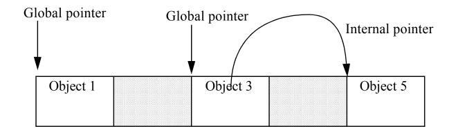
Objects 1 and 3 are marked because they are pointed to by global pointers. Object 5 is marked because it is pointed to by object 3, which is marked. Shaded objects are not marked and will be added to the free-space list.
