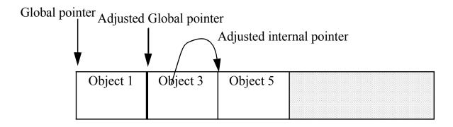
Compaction merges together freed objects into one large block of free heap space. Fragments are no longer a problem.
