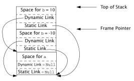
As usual, dynamic links always point to the next frame down in the stack. Static links always point down, but they may skip past many frames. They always point to the most recent frame of the routine that statically encloses the current routine.
