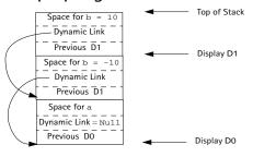
Since q is at nesting level 1, its frame is pointed to by D1. All of q's local variables, including b, are at a fixed offset relative to D1.
