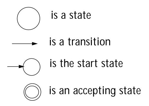
Finite automata (the plural of automaton is automata) are represented graphically using transition diagrams. We start at the start state. If the next input character matches the label on a transition
