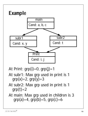
If A calls B (directly or indirectly), then none of A's register candidates are in the same group as any of B's register candidates.
