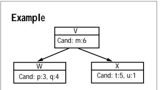
The algorithm can group candidate p with either t or u (since they don't interfere). It can also group candidate q with either t or u.
