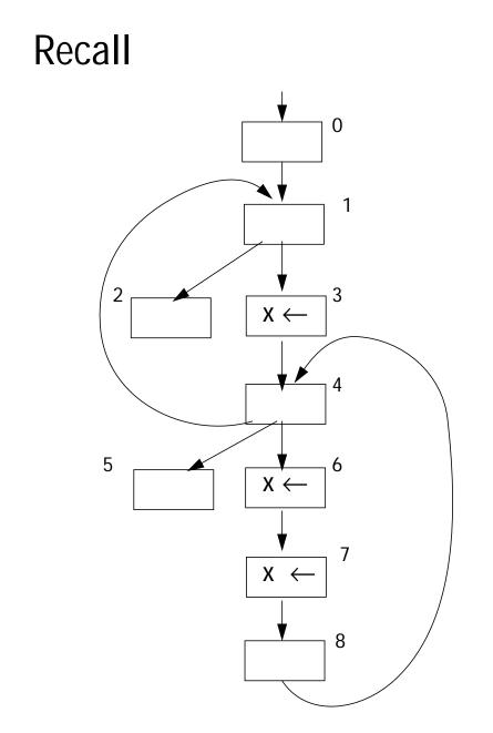
Here it took two passes to transmit the def in b7 to b1, so we expect 3 passes to evaluate *independent* of the lattice height.
