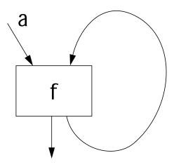
a is an input from outside the loop. Our concern is how often we'll need to reevaluate f, as new values are computed and fed back into f. Initially, we'll use T to model the value on the backedge. Iteration 1: Input =  $a \land T = a$ Output = f(a)Iteration 2: Input =  $a \land f(a)$ Output =  $f(a \land f(a))$ Iteration 3: Input =  $a \land f(a \land f(a))$
