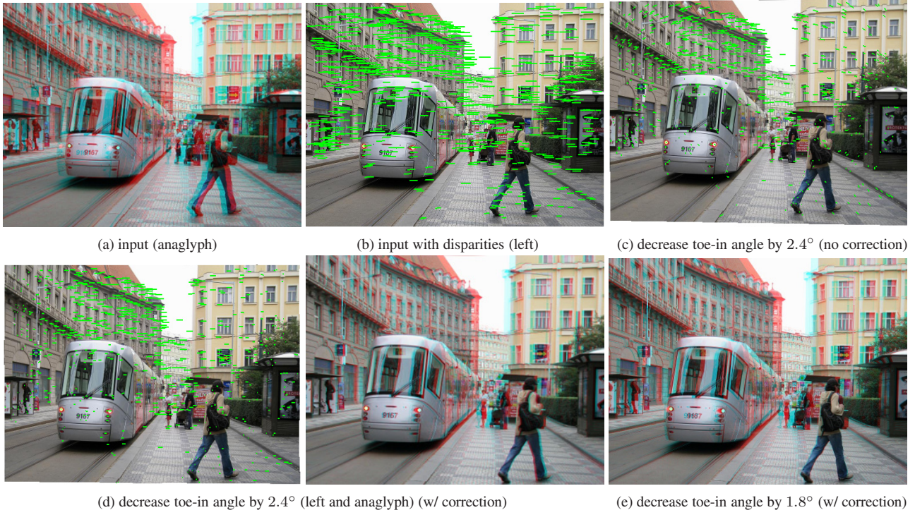
Figure 4. Decreasing the toe-in angle can move the train (d) or the person (e) near the screen. Toe-in angle change causes the keystone problem and introduces vertical disparities (c). Our method solves this problem (d, e).
