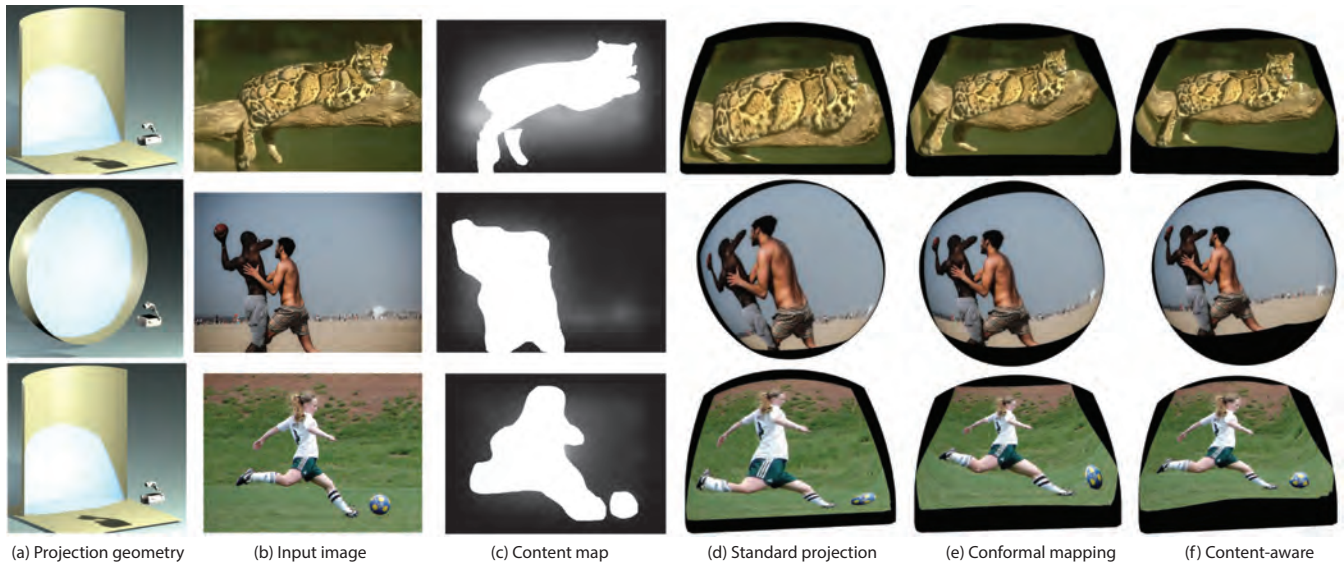
Figure 10: Examples of projection on non-developable surfaces. These examples show that our content-aware method can preserve the shape of the important image content well by distributing more projection distortion to less semantically important regions like sky, grassland, or blurry background.
