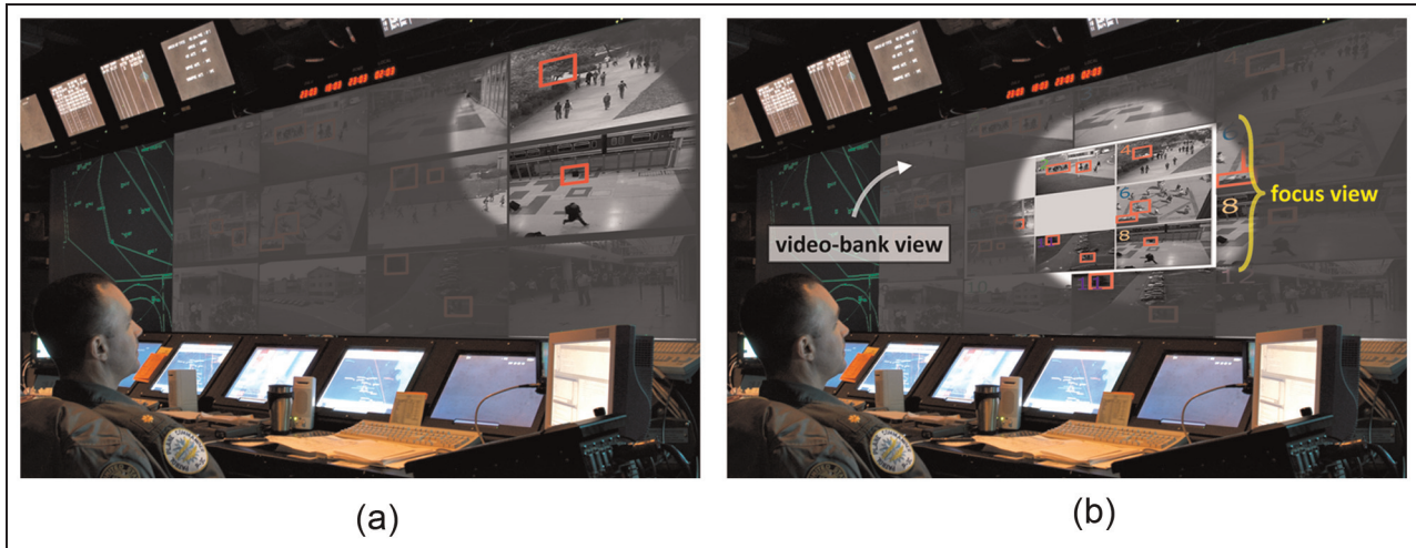
Figure 1. (a) Traditional computer vision-enabled surveillance system versus (b) Hotspot system. For illustration purpose only, the operator's attention focus region is highlighted as a bright circle and the screen outside the attention focus region is darkened. Using a traditional video surveillance system, an operator needs to shift his attention across the large display to cover/follow as many computer vision detected alarms as possible. This is cognitively demanding and often makes the operator miss important events. Hotspot summarizes the alarms in the focus view and allows the operator to quickly identify truly important events.
