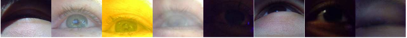
Fig. 2. Eye images captured by Smart Glasses in different lighting conditions. These images often have low quality and vary greatly from one another, clearly showing the need for a robust eye blink detection method.
