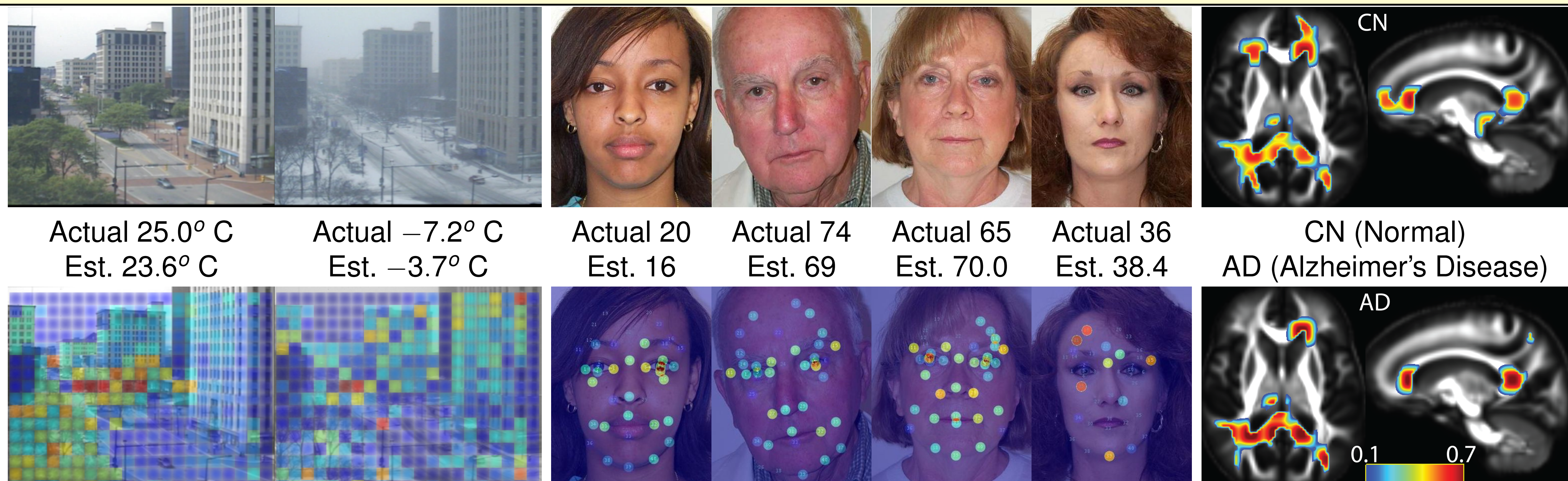
Figure: Dynamic feature weights for three tasks: ambient temperature prediction (left), age estimation (middle) on Lifespan database (Meredith et al., 2004, Guo, et al., 2012), and AD classification (right). AD classification accuracy of 86.17% by simple thresholding of continuous prediction by AIR comparing to SVM+PCA (80%-85%) (Hwang et al., 2015). AIR provides a way to determine, at test time, which features are most important to the prediction. Our results are competitive, which demonstrates that we achieve this capability without sacrificing accuracy.
