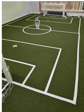
(b) The actual NAOv6 robot and soccer field used in the experiment. The robot perceives its environment through two head-mounted cameras, providing a field of view of 54.7^\circ .
