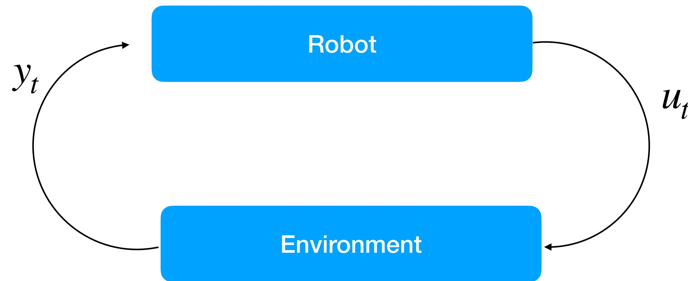
$$x_{t+1} \leftarrow F(x_t, u_t) \quad \text{or} \quad \begin{aligned} \dot{x}_t &\leftarrow F(x_t, u_t) \\ x_{t+1} &\leftarrow x_t + \dot{x}\Delta t \end{aligned}$$
