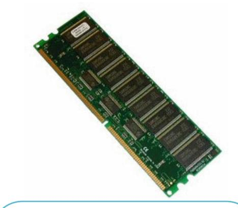
Servers are provisioned with 10s of GBS of memory and consume 30-57% of total power for a system provisioned with 128 GB DDR3 memory[2]
