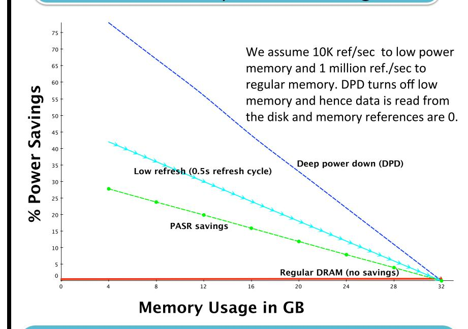
Result 2: Comparing power cost of copyout against savings from low power, we find mercurial caches can sustain a reference rate up to the row cycle time (~200K references)
