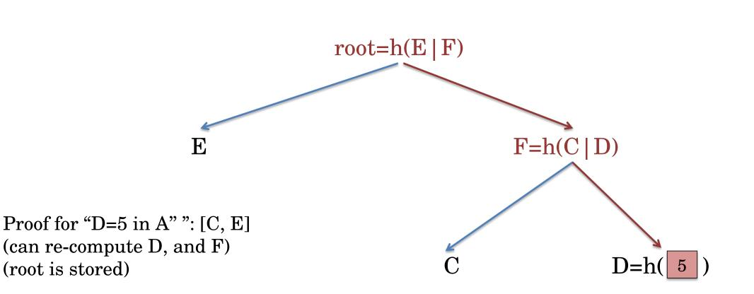
We can verify a single data item by comparing its branch with the root of the treeVerifier only needs to have the root stored
