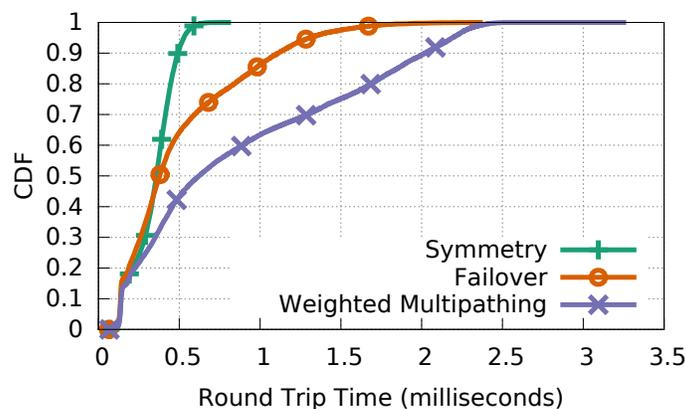
Figure 2.20: Presto’s RTT in symmetry, fast failover and weighted multipathing stages in random bijection workload.
