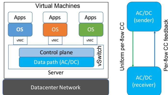
Figure 3.3: AC/DC high-level architecture.
