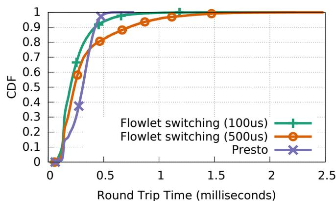
Figure 2.13: Round trip time comparison of flowlet switching and Presto in Stride workload. The throughputs of Flowlet switching with 100  $\mu$ s gap, 500  $\mu$ s gap and Presto are 4.3 Gbps, 7.6 Gbps and 9.3 Gbps respectively.
