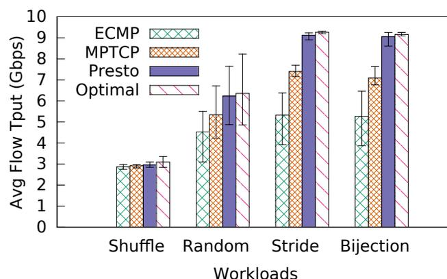
Figure 2.15: Elephant flow throughput for ECMP, MPTCP, Presto and Optimal in shuffle, random, stride and random bijection workloads.
