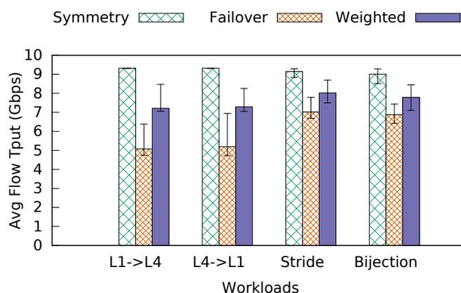
Figure 2.19: Presto’s throughput in symmetry, failover and weighted multipathing stages for different workloads.
