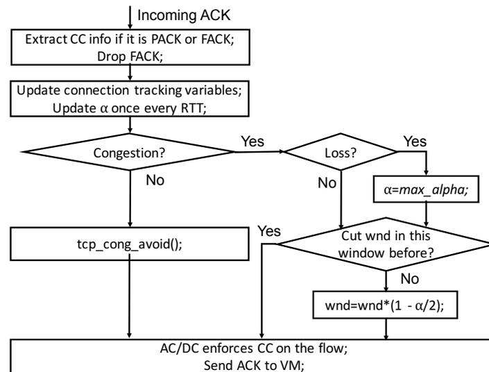
Figure 3.5: DCTCP congestion control in AC/DC.
