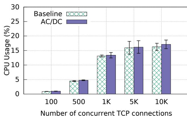
Figure 3.12: CPU overhead: receiver side (1.5KB MTU).
