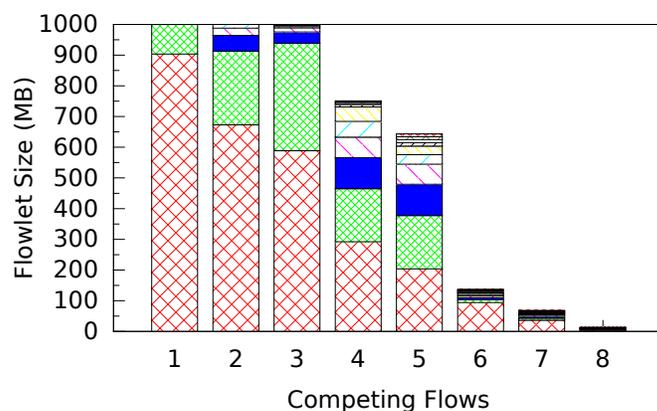
Figure 2.1: Stacked histogram of flowlet sizes (in MB) for a 1 GB scp file transfer. We vary the number of nuttcp [94] background flows and denote them as *Competing Flows*. The size of each flowlet is shown within each bar, and flowlets are created whenever there is a 500  $\mu$ s delay between segments. The top 10 flowlet sizes are shown here. We also analyzed the results of a 1 GB nuttcp, ftp, and a simple custom client/server transfer and found them to be similar.
