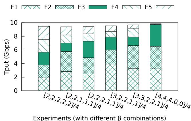
Figure 3.13: AC/DC provides differentiated throughput via QoS-based CC.  $\beta$  values are defined on a 4-point scale.
