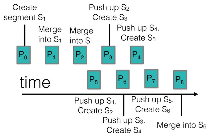
Figure 2.2: GRO pushes up small segments ( $S_i$ ) during reordering.
