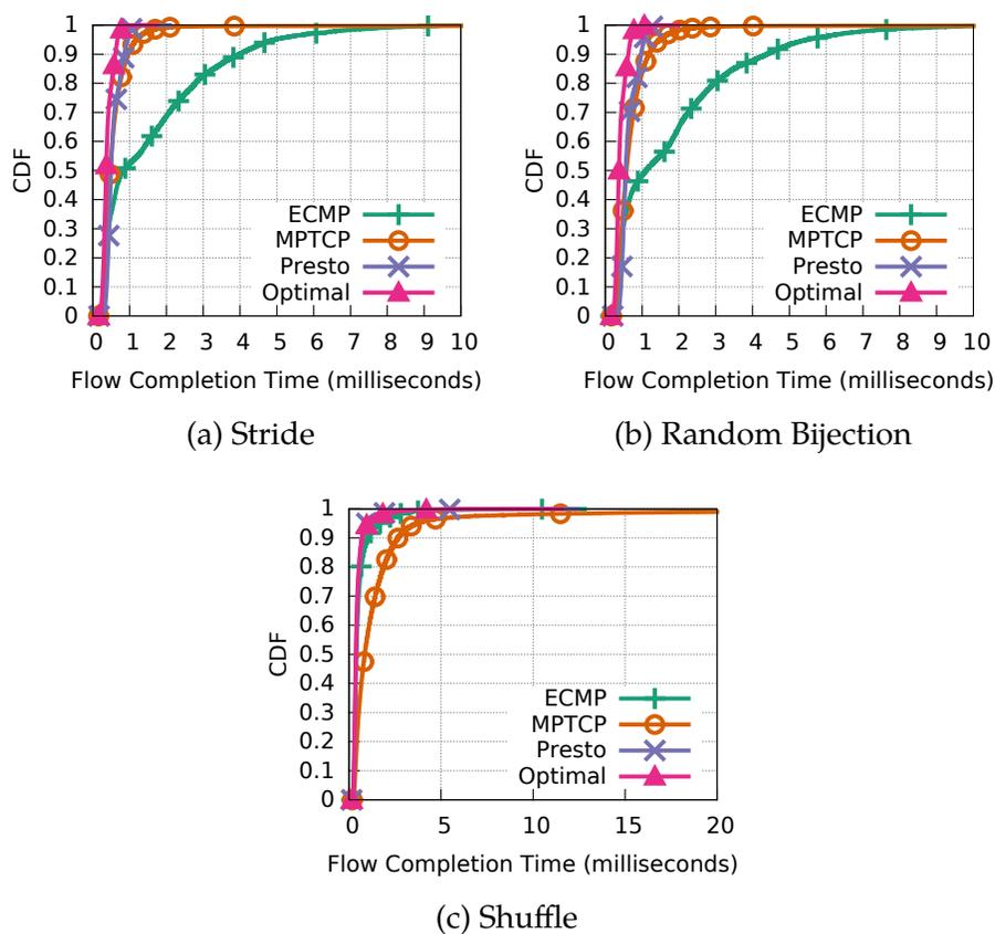
Figure 2.16: Mice FCT of ECMP, MPTCP, Presto and Optimal in stride, random bijection, and shuffle workloads.
