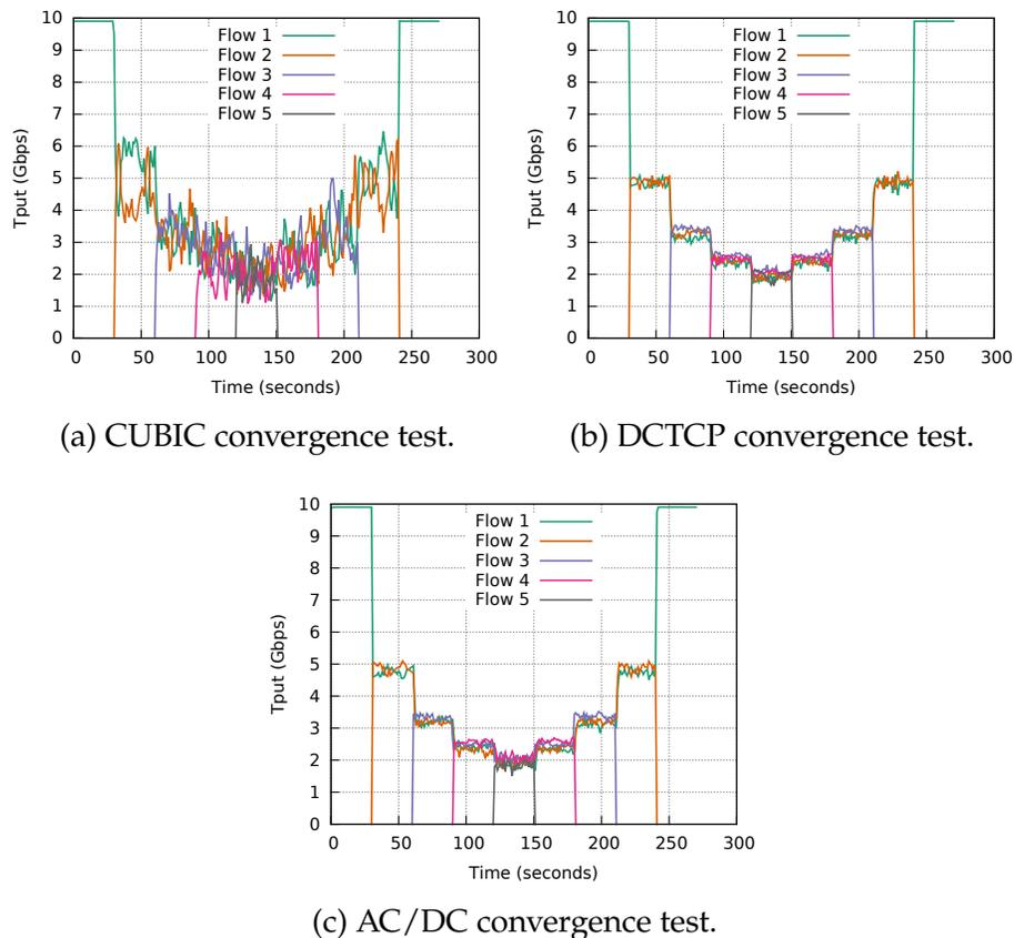
Figure 3.15: Convergence tests: flows are added, then removed, every 30 secs. AC/DC performance matches DCTCP.
