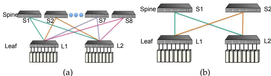
Figure 2.4: (a) Scalability benchmark and (b) Oversub. benchmark topology.
