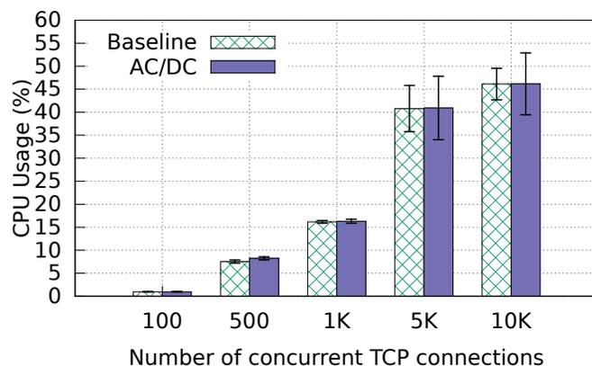
Figure 3.11: CPU overhead: sender side (1.5KB MTU).
