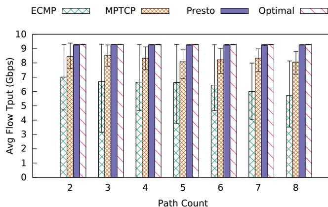
Figure 2.7: Throughput comparison in scalability benchmark. We denote the non-blocking case as Optimal.
