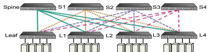
Figure 2.3: Our testbed: 2-tier Clos network with 16 hosts.
