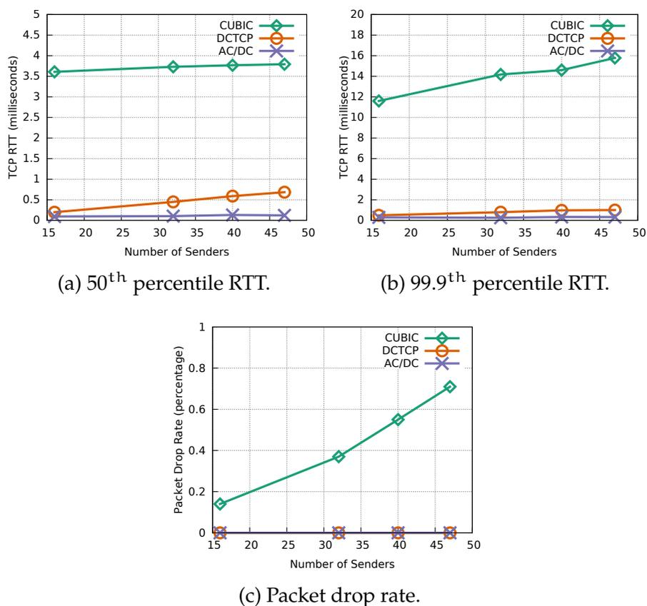
Figure 3.20: Many to one incast: RTT and packet drop rate. AC/DC can reduce DCTCP's RTT by limiting window sizes.
