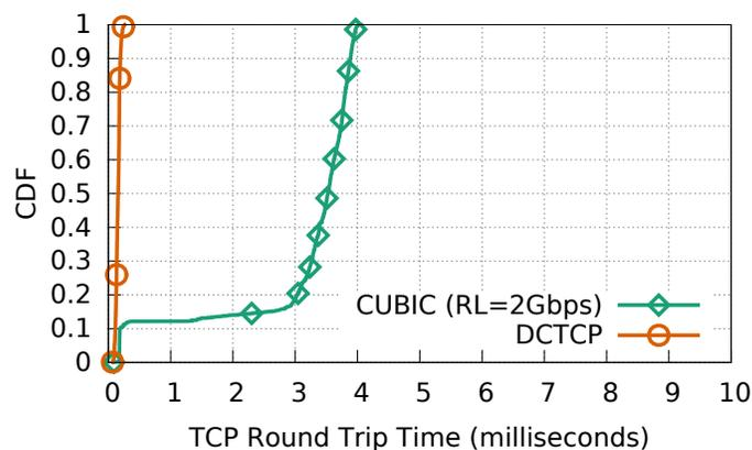
Figure 3.2: CDF of RTTs showing CUBIC fills buffers.
