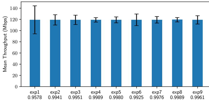
Figure 4.11: SPRING throughput fairness: 9 runs, 8 flows per run, rate-limiting=1Gbps, fairness index at the bottom
