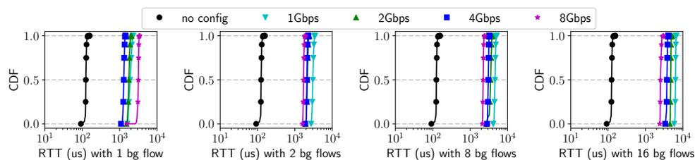
Figure 4.4: HTB experiment: one receiver VM, varying rate limiting and number of background flows
