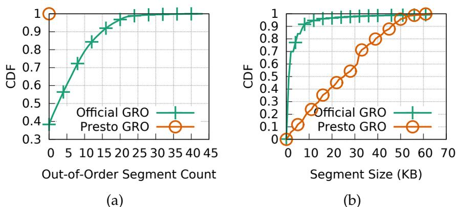
Figure 2.5: (a) Illustration of the modified GRO's effectiveness on masking reordering. (b) In case of massive packet reordering, official GRO cannot merge packets effectively such that lots of small packets are processed by TCP which poses great processing overhead for CPU.
