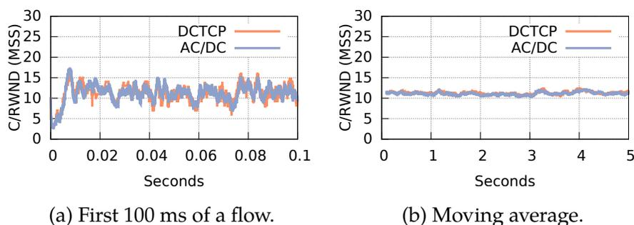
Figure 3.9: AC/DC's RWND tracks DCTCP's CWND (1.5KB MTU).
