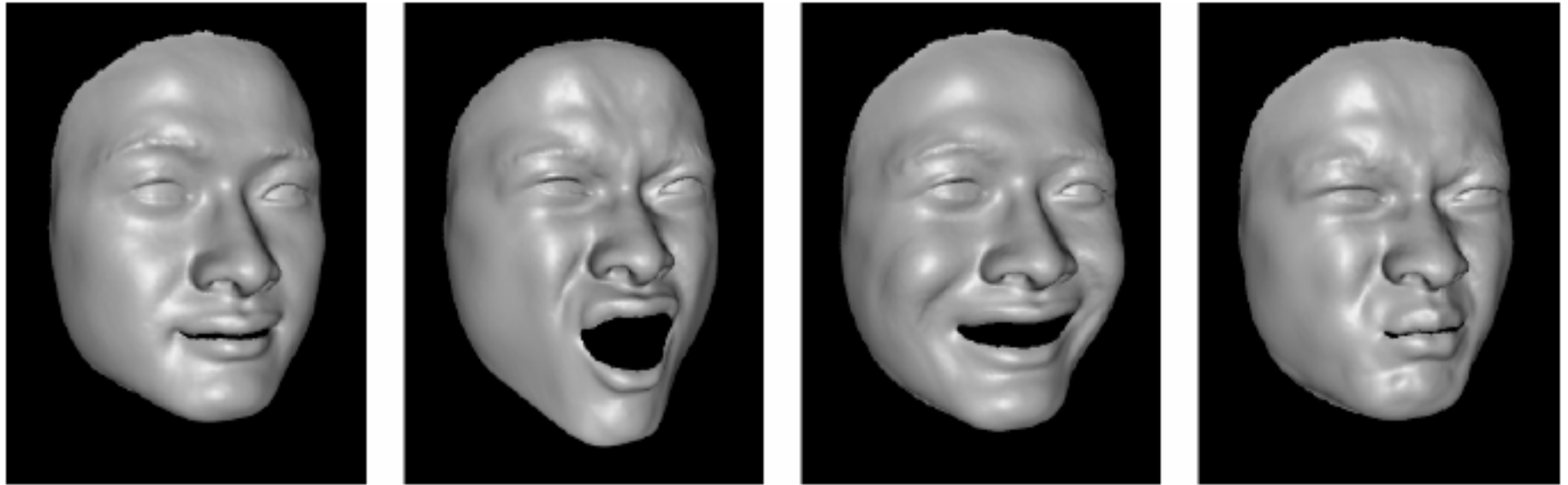
Four examples of recovered 3D shapes of a moving face from six video streams
