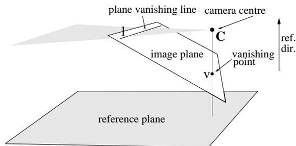
*Fig. 2. Basic geometry:* The plane’s vanishing line  $l$  is the intersection of the image plane with a plane parallel to the reference plane and passing through the camera centre  $C$ . The vanishing point  $v$  is the intersection of the image plane with a line parallel to the reference direction through the camera centre.
