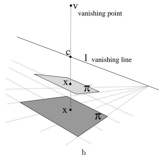
*Fig. 3. Distance between two planes relative to the distance of the camera centre from one of the two planes:* (a) in the world; (b) in the image. The point  $x$  on the plane  $\pi$  corresponds to the point  $x'$  on the plane  $\pi'$ . The four aligned points  $v, x, x'$  and the intersection  $c$  of the line joining them with the vanishing line define a cross-ratio. The value of the cross-ratio determines a ratio of distances between planes in the world, see text.
