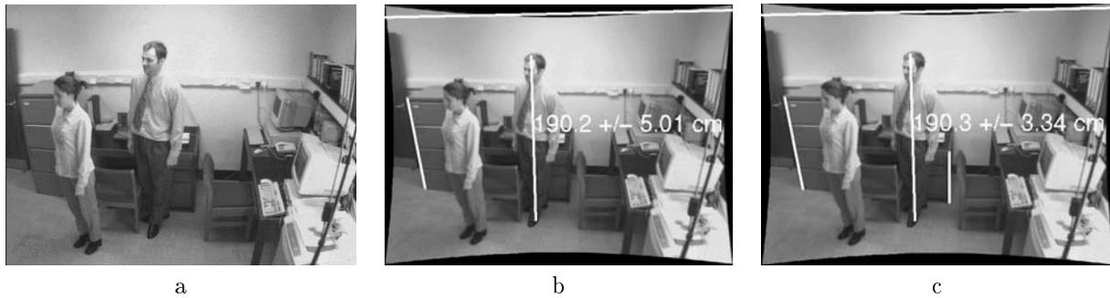
**Fig. 17. Measuring heights and estimating their uncertainty, second point of view:** (a) Original image; (b) the image has been corrected for radial distortion and height measurements computed and superimposed. With *one* supplied reference height  $Z = 190.2 \pm 5.01$ cm (*c.f.* ground truth value 190cm). (c) With *two* reference heights  $Z = 190.3 \pm 3.34$ cm. See figure 16 for details.
