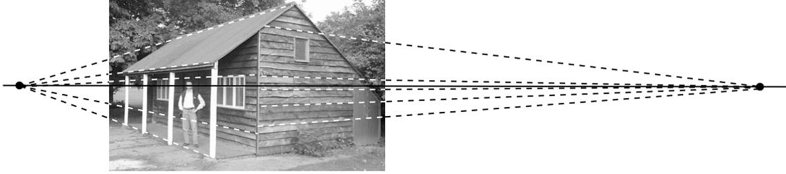
*Fig. 24. Computing the plane vanishing line:* The vanishing line for the reference plane (ground) is shown in solid black. The planks on both sides of the shed define two sets of lines parallel to the ground (dashed); they intersect in points on the vanishing line.
