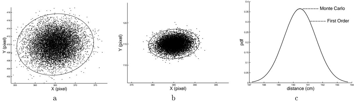
*Fig. 19. Monte Carlo simulation of the example in fig. 16d:* (a) distribution of the input base point  $\mathbf{x}$  and the corresponding 3-standard deviation ellipse. (b) distribution of the input top point  $\mathbf{x}'$  and the corresponding 3-standard deviation ellipse. Note that figures (a) and (b) are drawn at the same scale. (c) the analytical and simulated distributions of the computed distance  $Z$ . The two curves are almost perfectly overlapping.
