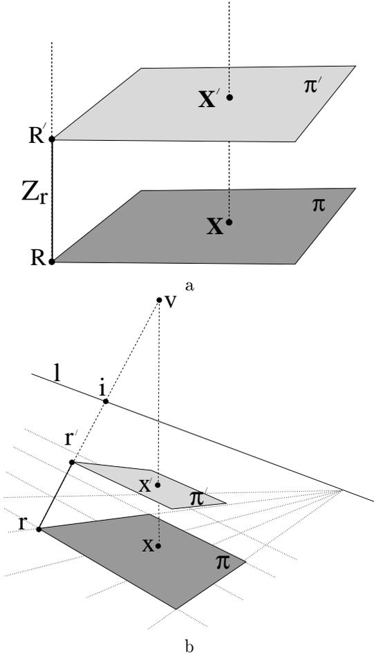
*Fig. 7. Homology mapping between imaged parallel planes:* (a) A point  $X$  on plane  $\pi$  is mapped into the point  $X'$  on  $\pi'$  by a parallel projection. (b) In the image the mapping between the images of the two planes is a homology, where  $v$  is the *vertex* and  $l$  the *axis*. The correspondence  $r \rightarrow r'$  fixes the remaining degree of freedom of the homology from the cross-ratio of the four points:  $v$ ,  $i$ ,  $r'$  and  $r$ .
