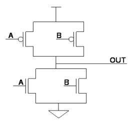
There is short circuit (path from Power to Ground) when either A = 1 and B = 0 or A = 0 and B = 1.
