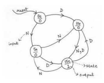
II. How many flip-flops (storage elements) will be needed to implement this finite state machine designed in your answer to part I?
