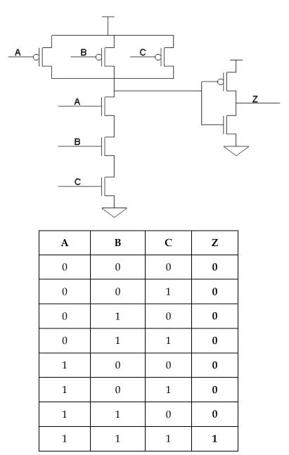
**Note:** This is the truth table for AND gate, if you did the truth table for a NAND gate overlooking the inverter, you received partial credit.
