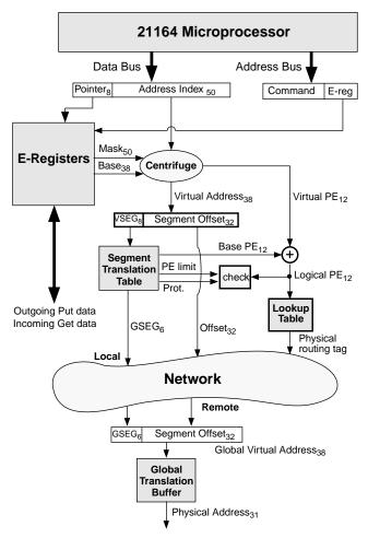
Figure 4. Address translation for global (E-register) references
