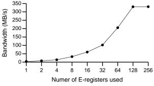
Figure 7. Effect of pipelining in the memory interface
