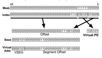
Figure 3. HW centrifuge operation example: Array interleaved by cache line over 64 PEs
