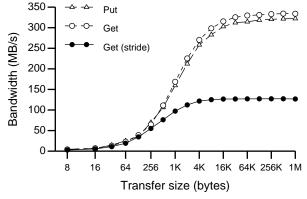
Figure 8. Effect of startup latency on realized bandwidth
