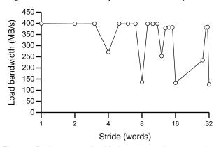
Figure 9. Performance of strided memory references using E-registers
