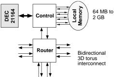
Figure 1. T3E PE block diagram
