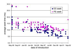
Figure 7: Comparison of seek times [Seagate02].
