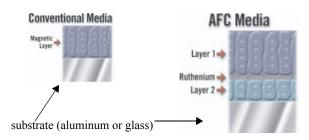
Figure 3: Diagram of media layers. The base substrate consists of either aluminum or glass, topped with a layer of magnetic material. In anti-ferromagnetically coupled (AFC) media, an additional layer of magnetic material and a layer of ruthenium are added, with the two layers reinforcing each other for better magnetic stability at higher density.
