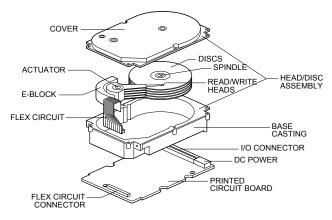
Figure 2: Diagram of the major components of a disc drive.
