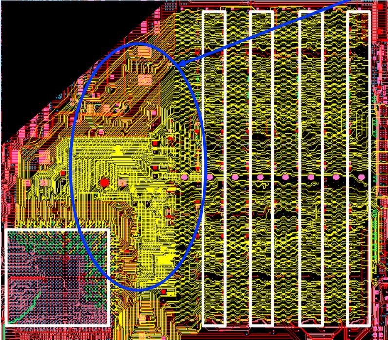
Serpentine routing is complicated and uses up a lot of board area
