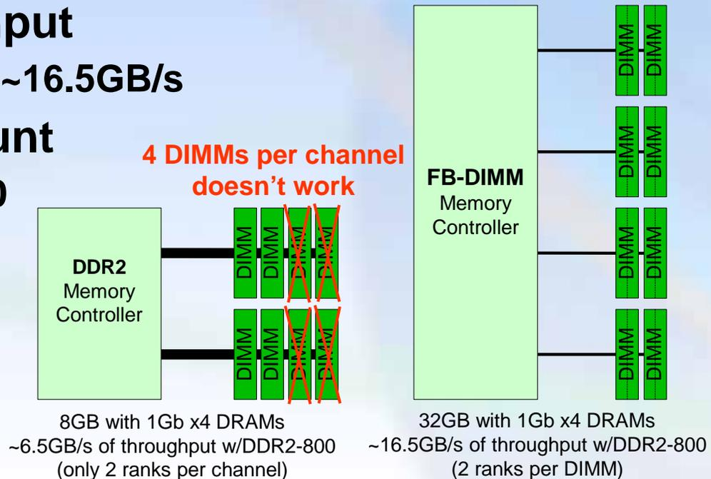
**FB-DIMM Provides 4x the Capacity**
