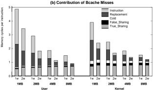
Figure 5: OLTP execution time (a) and Bcache behavior (b) for different cache sizes and associativity (P=4).
