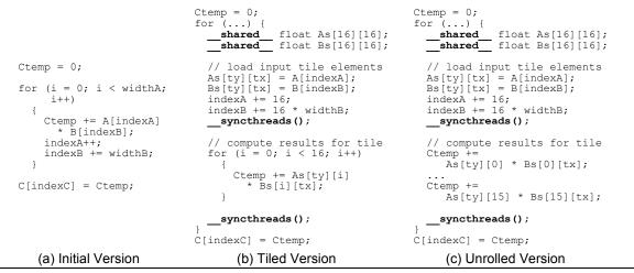
Figure 3. Partial Kernel Codes for Matrix Multiplication. CUDA keywords are bold.
