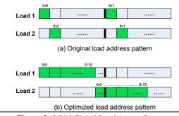
Figure 5. LBM Global Load Access Patterns
