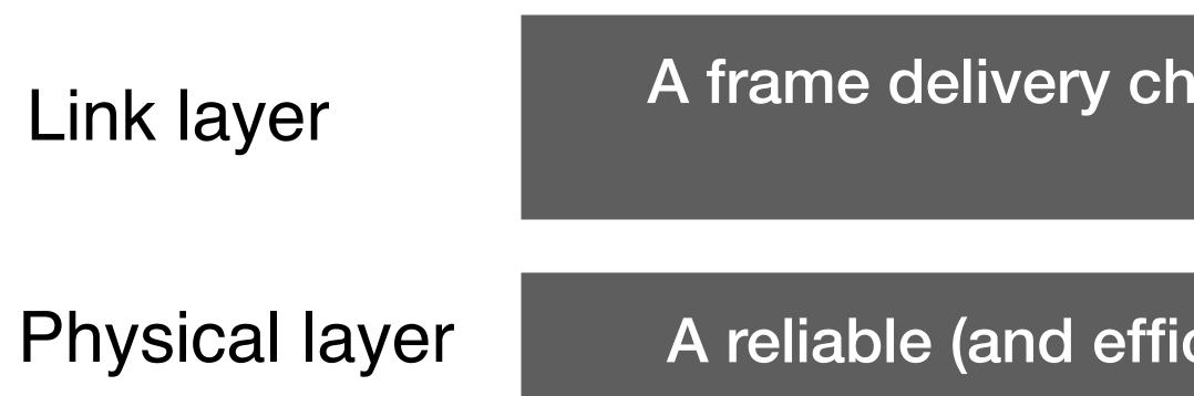
A frame delivery channel between directly connected or switched hosts
