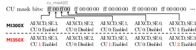
Figure 15: Reverse-engineered MI300X/MI350X CU mask.
