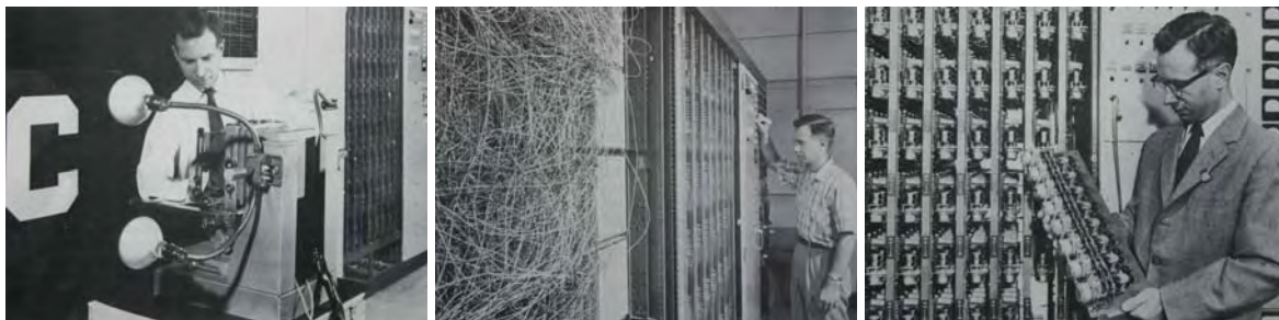
Figure 4.8 Illustration of the Mark 1 perceptron hardware. The photograph on the left shows how the inputs were obtained using a simple camera system in which an input scene, in this case a printed character, was illuminated by powerful lights, and an image focussed onto a 20 \times 20 array of cadmium sulphide photocells, giving a primitive 400 pixel image. The perceptron also had a patch board, shown in the middle photograph, which allowed different configurations of input features to be tried. Often these were wired up at random to demonstrate the ability of the perceptron to learn without the need for precise wiring, in contrast to a modern digital computer. The photograph on the right shows one of the racks of adaptive weights. Each weight was implemented using a rotary variable resistor, also called a potentiometer, driven by an electric motor thereby allowing the value of the weight to be adjusted automatically by the learning algorithm.
