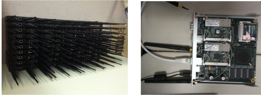
Figure 2.2: We built the WiSe Access Point platform using OpenWrt based APs (left). Each WiSe Access Point consists of two WiFi cards (right). The primary card acts as an Access Point to serve WiFi client devices in homes and also capture different channel and link related parameters. The secondary WiFi card is used for additional passive wireless measurements.
