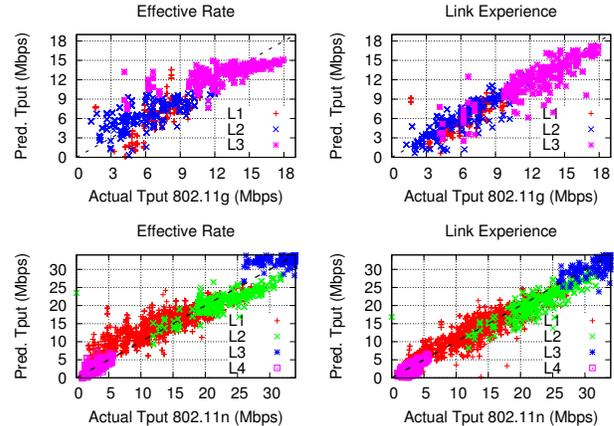
**Figure 4: Scatter plot showing the actual vs. predicted TCP throughput values for the 802.11g (top) and 802.11n (bottom) ground truth experiments by using "Effective Rate" and "Link Experience". Points near the "x=y" line indicate instances with accurate prediction of TCP throughput. Each set of points corresponds to a different WiFi link.**
