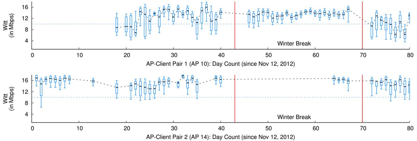
**Figure 8: Distribution of Witt for 2 different AP-client pairs in our deployment from 12 Nov 2012 to Jan 31, 2013 and shows their variation in performance over the span of this period. 10th, 25th, 50th, 75th and 90th percentiles are shown in this figure.**
