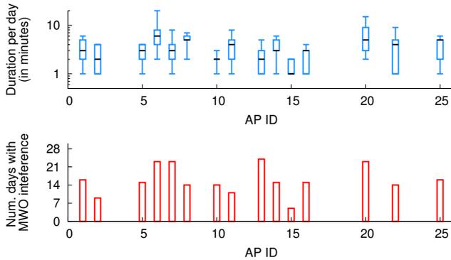
**Figure 13: (top) Distribution of duration per day during which microwave interference reduced Witt by 20%. (bottom) Number of days from a 30 day period, during which the APs experienced at least 1 minute of such interference.**
