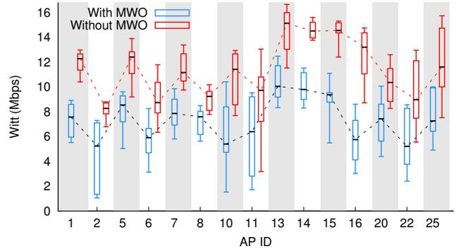
**Figure 14: Candlestick plot comparing the estimated average Witt for WiSe APs with active WiFi links during and after the completion of microwave oven activity. 10th, 25th, 50th, 75th and 90th percentiles are shown in this figure. The dotted line compares the 50th percentile values for both cases.**
