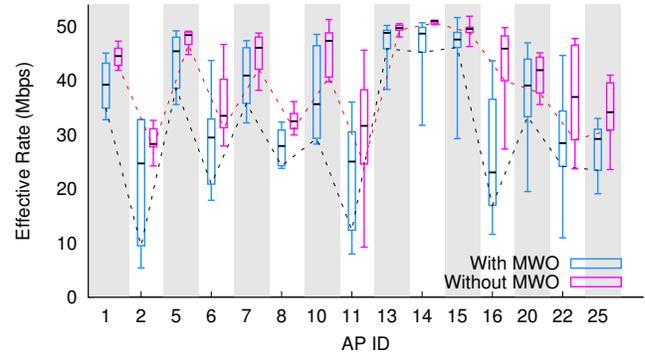
**Figure 15: Candlestick plot comparing the airtime utilization (left) and effective rates (right) for WiSe APs with active WiFi links with and without microwave oven interference. 10th, 25th, 50th, 75th and 90th percentiles are shown in this figure. The dotted line compares the 25th and 75th percentile values for airtime utilization and effective rate respectively.**
