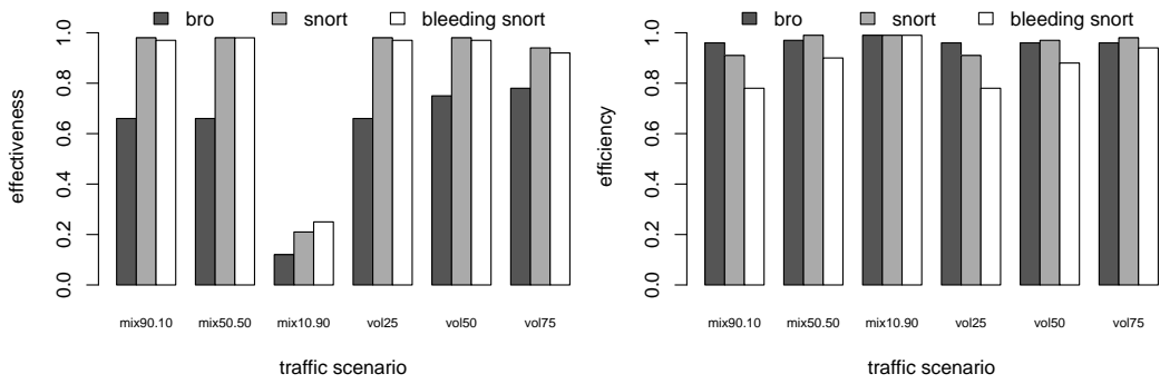
Figure 7: Alarm effectiveness (left) and efficiency (right) for Bro, Snort, and Bleeding Snort on CSL traffic setup.
