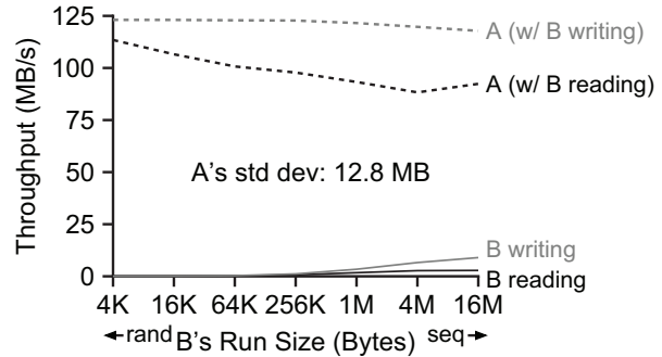
Figure 16: Isolation: Split-Token with XFS. This is the same as Figure 6 and Figure 14, but for XFS running with our Split implementation of token bucket.
