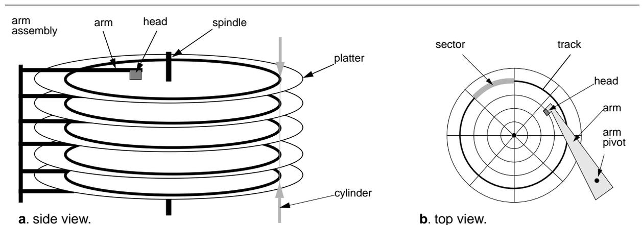
**Figure 1:** the mechanical components of a disk drive.
