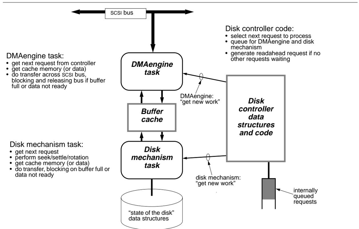
**Figure 3:** simulation model structure for a single disk.
