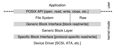
Figure 36.4: The File System Stack
