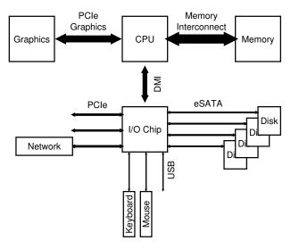
Figure 36.2: Modern System Architecture
