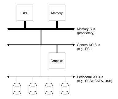
Figure 36.1: Prototypical System Architecture
