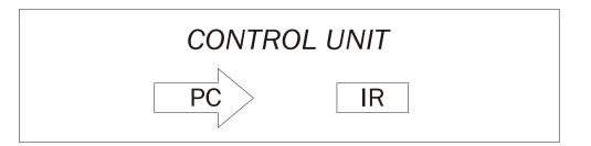
Instruction Register (IR) contains the <u>current instruction</u>. Program Counter (PC) contains the <u>address</u> of the next instruction to be executed.
