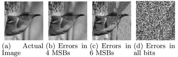
**Figure 4: Effect of random errors at different bit-pairs of a representative BMP image**
