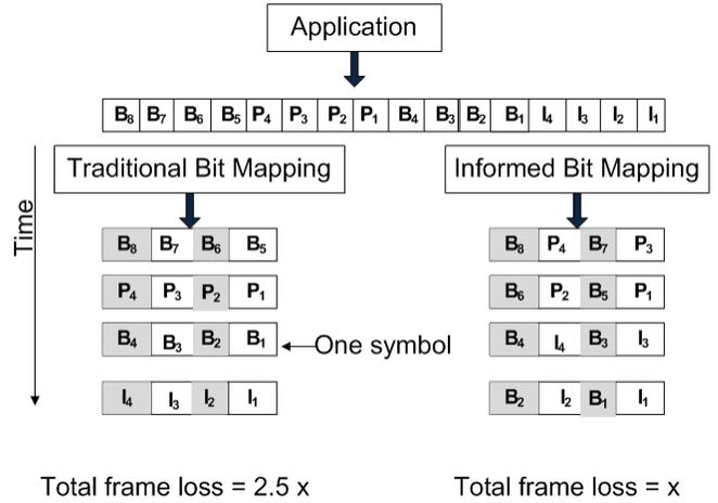
Figure 6: Informed bit mapping for bit error differentiation.
