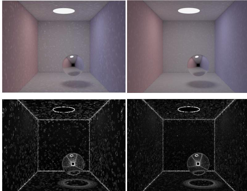
**Figure 4:** Results for MIS and OCV for irradiance caching computations on a box scene. Standard irradiance caching, which uses MIS for its estimates, is on the left, while a version using OCV estimators is on the right.
