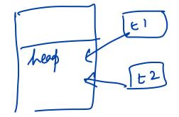
Can have multiple threads within a single process
