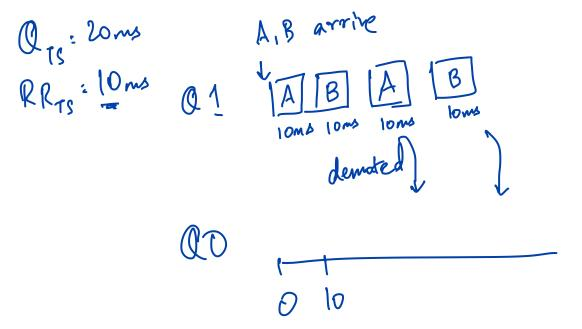
t. 10 ms A has used 10 ms At < Q<sub>Ts</sub> Keep A at 01
