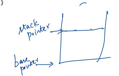
%**rbp** is the base pointer: points to base of current stack frame
