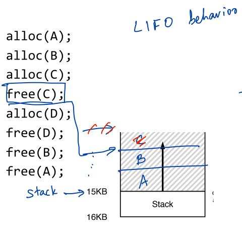
Pointer between allocated and free space Allocate: Increment pointer Free: Decrement pointer
