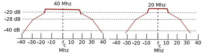
Figure 7: Transmit spectrum masks for 40 MHz and 20 MHz channels for the physical layer in IEEE 802.11n standard
