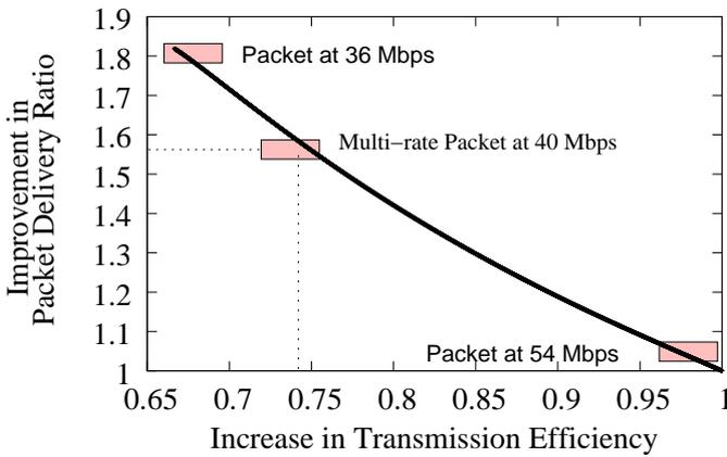
Figure 3: Tradeoff between transmission efficiency and packet delivery ratio for an 802.11 wireless channel. Multi-rate provides a continuum of data rates with different transmission efficiencies and packet delivery ratios to choose from.
