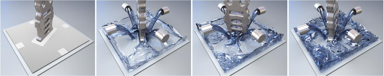
Fig. 3. Four sources pour water that collides with a kinematic rotating object in a container, with effective resolution  $512^3$ . The adaptivity pattern, illustrated on the left, continuously rotates with the central spinning object. A narrow band level set with  $2048^3$  resolution is used to track the free surface.
