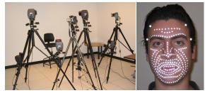
Figure 2: Eight camera optical motion capture layout (left), 250 facial marker set (right).
