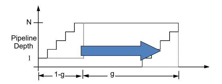
g = fraction of time pipeline is filled 1-g = fraction of time pipeline is not filled (stalled)
