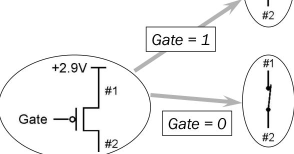
Terminal #1 must be connected to +2.9V.
