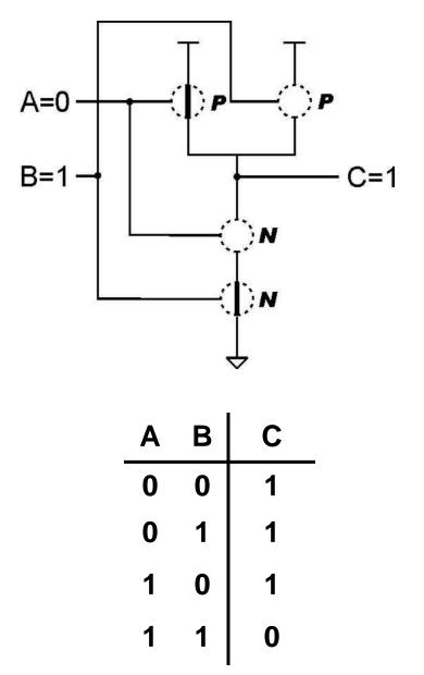
Note: Parallel structure on top, serial on bottom.
