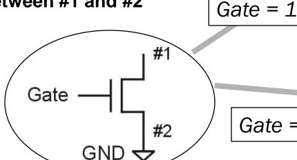
Terminal #2 must be connected to GND (0V).
