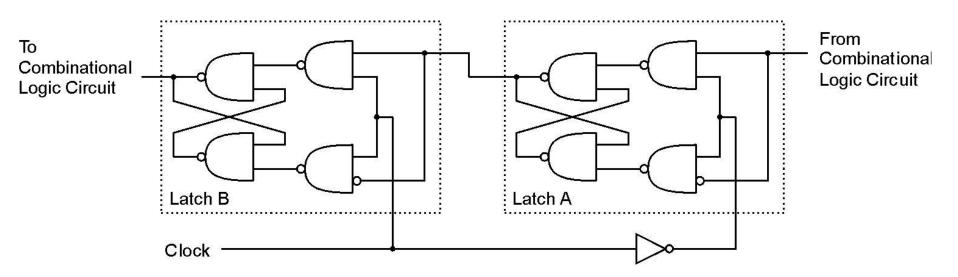
During 1<sup>st</sup> phase (clock=1), previously-computed state becomes *current* state and is sent to the logic circuit.
