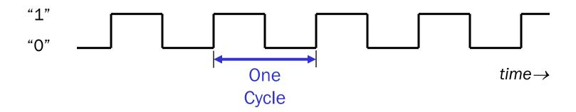
At the beginning of each clock cycle, state machine makes a transition, based on the current state and the external inputs.
