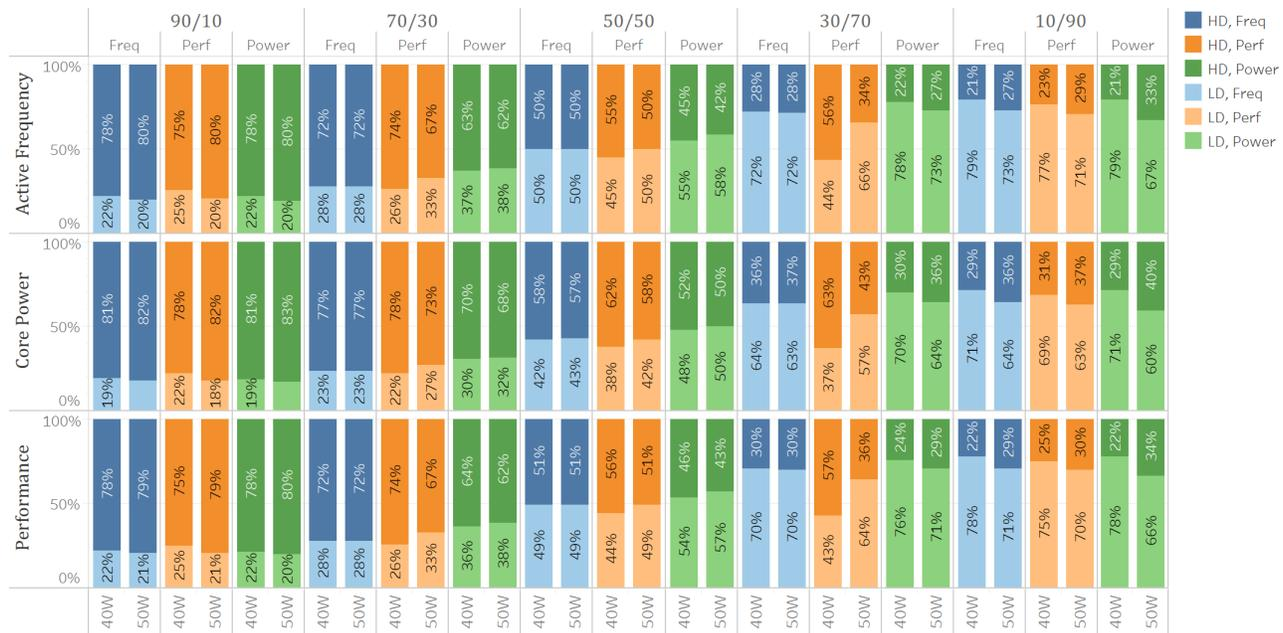
**Figure 10.** Ryzen proportional share policy experiments. The figure shows percent of total resource used by each application for frequency, performance, and power shares. Each pair of bars shows results for 40W and 50W limits. Each row represents the measured use of a different resource.
