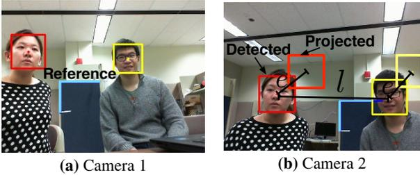
**Figure 7:** Two cameras simultaneously capture a scene containing the same two faces. To avoid redundant counting, Vigil projects faces from Camera 1 to Camera 2 based on common reference points denoted by the two blue lines labeled “Reference” in Camera 1’s view. If projection error does not exceed the distance between the detected faces, re-identification correctly identifies the two views of each face.
