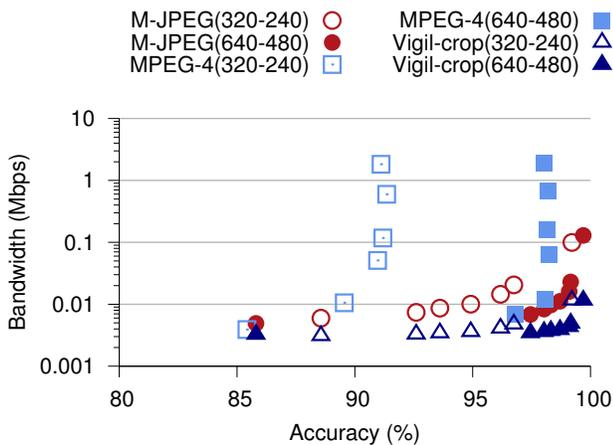
**Figure 18:** Bandwidth required versus accuracy of the face detection vision algorithm on videos compressed with different video compression algorithms, including our algorithm Vigil-crop that performs M-JPEG on the cropped objects. Only the selected frames in the `sis` array are compressed for this bandwidth calculation.
